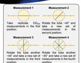
Figure 3: The illustration shows the above view of a test tube and how it can be rotated between replicate measurements to minimise the effects or irregular refraction.
