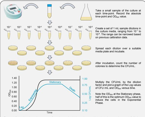
Figure 4: Illustration shows the process of creating a microbial growth curve. Note that when creating a set of dilutions, performing serial dilutions should be avoided as they are inherently inaccurate.
