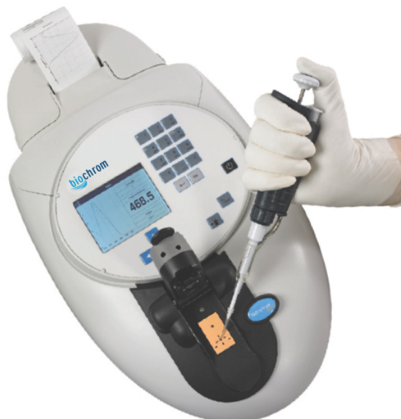
Fig 1. The NanoVue Plus Spectrophotometer uses a novel drop-and-measure sample plate which eliminates the need for cuvettes.
